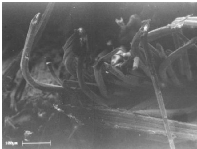
Figure 6 Scanning electron micrograph of a 20% alkali treated bamboo fiber-resol resin composite.
